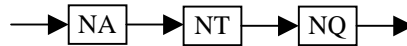
Figure 8.C.8 — Noise processing blocks. NA = Noise analysis, NT = Noise temporal envelope and NQ = Noise quantization
